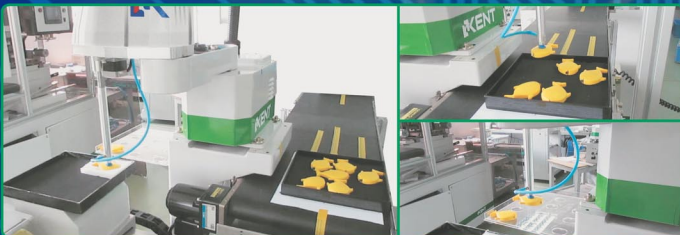
Release and pick by vision system
