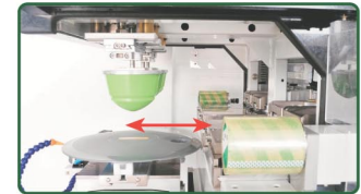
Pad in/out stroke for max. throat depth
