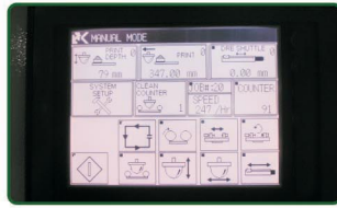
PLC touch screen control
