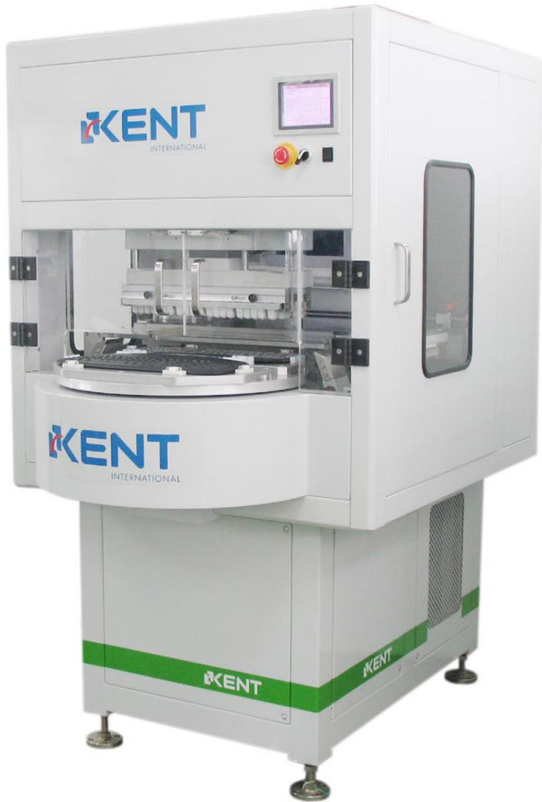
2007 Servo Motor Keyboard Printing System (No Product Mask)
